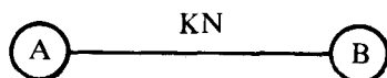
Figure 4-13. Shorthand Notation Representing Key Protection Between Nodes A and B Using Secondary Key KN
